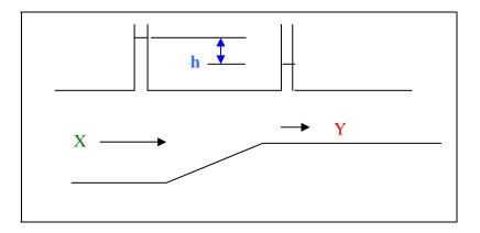
Equation of continuity  $A_X V_X = A_Y V_Y$  .....(1) Bernoulli's equation  $P_X + \rho V_X^2/2 = P_Y + \rho V_Y^2/2$ i.e.  $P_X - P_Y = \rho V_Y^2/2 - \rho V_X^2/2$  .....(2) Eliminate  $V_Y$  (or  $V_X$ ) from (1) and (2) http://phy.hk
