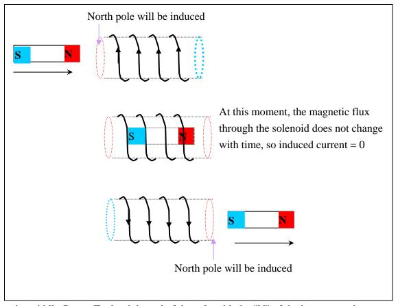
More about the middle figure: To the right end of the solenoid, the "N" of the bar magnet is approaching, so a north pole is induced there.
