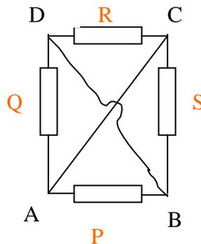
Current enters A -----pass through P (A to B)-----exit at B, or
