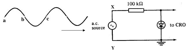
1. The diode is assumed ideal, i.e. resistance of the diode = 0 (perfect conductor) when the diode is forward-biased.
