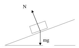
The acceleration is horizontal, so upward force = downward force
