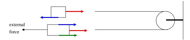
Red force: tension = T (along the same string, tension is unchanged)
